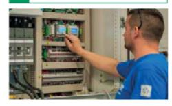
Once completed the refrigeration and water circuit, we perform the electrical wiring and the connection between electric board and compressor, fan, pump, etc. .Each unit is equipped with electric panel, built, wired and fully tested at the factory. Wiring numeration and optimized layout facilitate troubleshooting. The installed components are identified by nameplates to better identify the application and the type of action.
