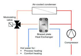
The solution proposed by Euroklimat for Total Heat Recovery is a modulating solution, based on the concept that the recovery load may vary during the function of the unit and, as a consequence, there could be:
